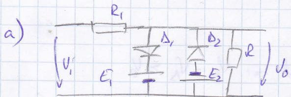
$$\begin{aligned} D_1 \text{ d } &\Leftrightarrow V_o - V_d \geq E_1 \\ D_2 \text{ d } &\Leftrightarrow V_o + V_d \leq -E_2 \end{aligned} \quad \left\{ \Rightarrow V_o \in [-E_2 - V_d, E_1 + V_d] \text{ am beide diode } \rightarrow \text{feste} \right.$$
