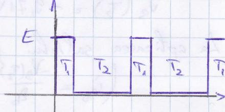
$$V_{cc} = 15V, T_2 = 4T_1 \approx 10\mu s$$
