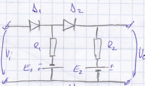
$$a) \quad V_d = 0.8V, \quad R_1 = R_2 = 1k\Omega, \quad E_1 = E_2 = 5V$$
