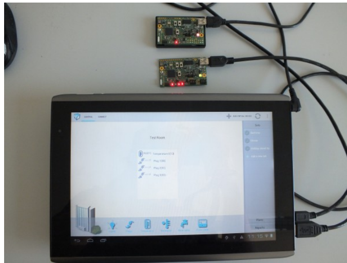
Figure 4.4: Test with a client device. The test dongle (right on top of the tablet) uses the same platform as the network device (top board).
