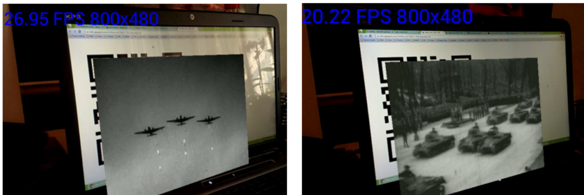
Figure 4.8: Application screenshots, while displaying historical video clips on top of a QR code shown on a screen.
